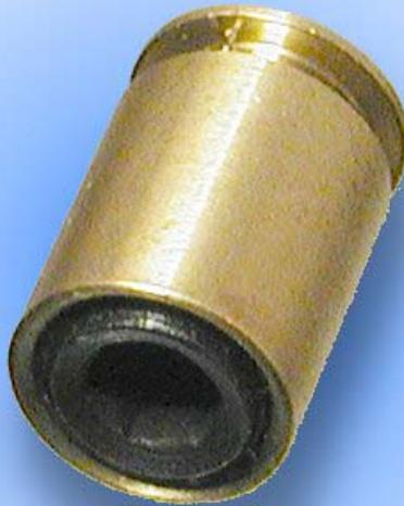
The Regulator Piston comes as an assembly. DO NOT take this apart. It has a built in blow off valve that will leak air if your marker becomes over pressurized. The blow off resets once your pressure goes back to normal. This safety feature is found exclusively in AGD markers. Replace the entire assembly if your marker is shooting at normal speeds and it still leaks out the back.
