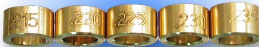
The PT Spacer Kit gives you five different brass spacers all legibly numbered so you can adjust the spacing of the power tube o-ring. If your marker has bolt stick use a longer one, if it leaks down the barrel use a shorter one. Find one that works and stick with it! Quality machined brass to AGD standards. PT Spacer Kit comes with an extra power tube o-ring not shown.
