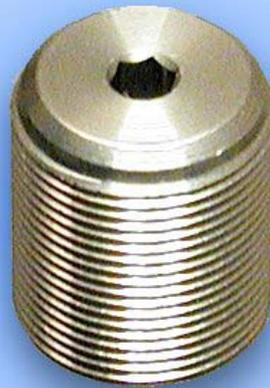
The very back of the marker has this adjustment nut to change your velocity. Made from high quality stainless steel. Use a high quality grease on the threads to reduce galling.
