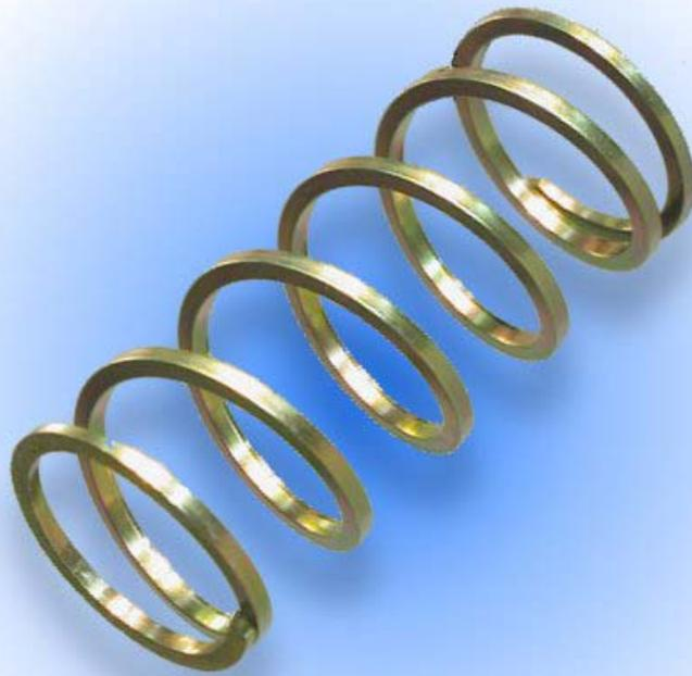
The Bolt Spring fits all AGD markers regardless of age or type. They are made from very special square wire so they don't fold inside themselves when collapsed. Replace your old springs when they sag below the front of the bolt. Special honed bolt springs come with Superbolts to prevent premature wear. One spring also comes in the Parts Kit. If you need any o-rings the kit is a good value.
