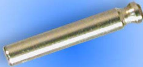
The On/Off Pin controls air flow in your marker. It is a critical precision component and should not be modified. It's hardened and chrome plated for extra long life.
