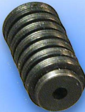
Not usually something that wears out. The Spring Pack comes as an assembly with all the disk springs organized in a special way. DO NOT try to take it apart! Keep it clean and lightly greased.
